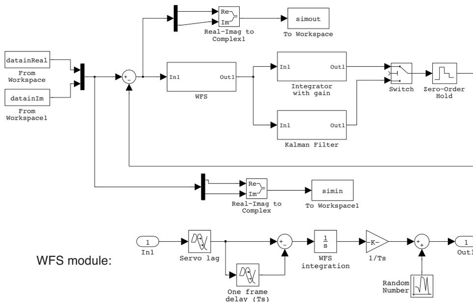
Fig. 4. Simulink model of the hybrid continuous-time/discrete-time AO control loop for a complex-valued Fourier modal coefficient. The WFS module implements the standard transfer function  $W(s)$ , while the DM module is a Simulink zero-order hold block. The integral controller and Kalman filters are implemented with discrete-time blocks of gains and delays. (The Kalman block is implemented exactly as in Fig. 3.) A switch allows use of either controller.
