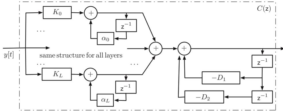
Fig. 3. Flow diagram illustrating the implementation of the predictive filter for  $0 \leq \tau \leq 2T$ . The coefficients used in the filter depend on  $\Delta$  and are taken from Eqs. (39)–(41). Note that when  $\tau \leq T$ ,  $D_2=0$ .
