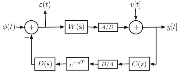
Fig. 1. Block diagram of hybrid continuous-time/discrete-time AO control loop for a single Fourier mode. The phase aberration  $\phi(t)$  is corrected in closed loop in the presence of measurement noise  $v[t]$ . The WFS dynamics are represented by  $W(s)$ , the DM dynamics by  $D(s)$ , and the controller delay by  $\exp(-s\tau)$ . The discrete-time control law is  $C(z)$ . A/D and D/A conversion surround the control computer.
