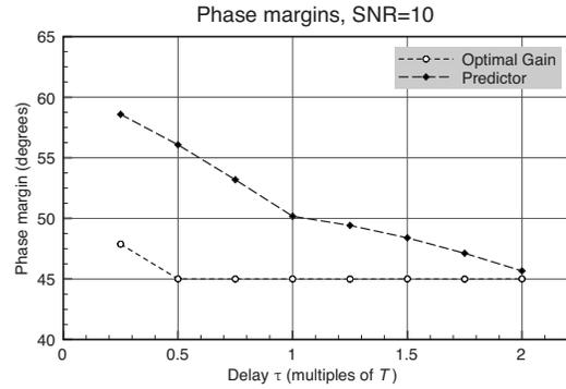
Fig. 6. Phase margins for a high-SNR case for the optimized-gain integrator and the predictor. For most delays  $\tau$ , the optimal gain is limited to be the maximum gain set by stability. The predictor can be more aggressive and has larger margins for all  $\tau$ . Note how the margin gracefully transitions between integer time step delays.
