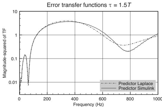
Fig. 5. Error transfer function for a predictive controller with  $\tau=1.5T$ , based on the Laplace transform model or as determined by running white noise through the Simulink model. There are some small discrepancies due to the modeling of the DM.
