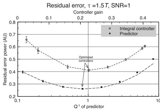
Fig. 7. Residual error performance of the integral controller and the predictive filter for a variety of gains. The optimized gain (as determined by Laplace analysis) results in the best performance in Simulink. The predictor was manipulated by feeding an incorrect WFS noise level into the ARE solve, producing a range of predictors. Again, the predictor produced by the model results in the best performance in Simulink.
