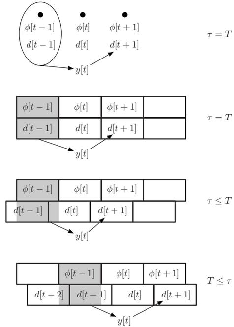
Fig. 2. Comparison of the discrete-time state space model for delay  $\tau=T$  (row 1) to the new model, which assumes the signals are constant over an interval of the sampling period (row 2). When  $\tau \leq T$ , the DM signal shifts to the left and becomes asynchronous (row 3). When  $T \leq \tau$ , the DM signal shifts to the right (row 4).
